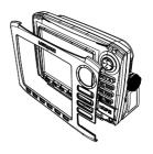
**9:** Attach the bezel. Firmly clip the front bezel in place.
